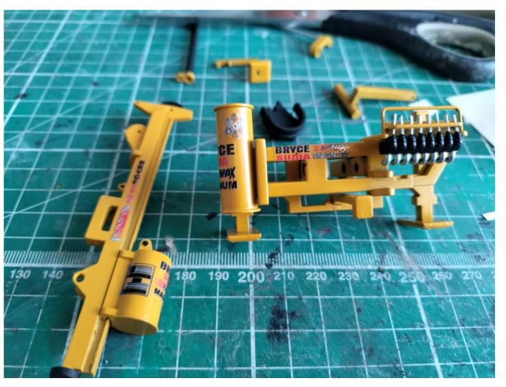
Step 26: Final assembly starts by attaching the rock spike holder to the main frame. To do this cut a short length of the 1mm wire supplied with the kit, bend one end over to make an L shape, thread the longer end through the mounting holes and bracket, then bend the other end over to lock the parts in place.
