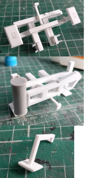
**Step 15:** Assemble the towbar bracket by gluing 24 to the front edge of 23 and gluing 23 in the slot on the main frame, glue the printed towball to the front of 24. The feet 10 can now be glued to the main frame. We have sanded a 45 degree chamfer on all four edges of the feet to look more like the real machine.
