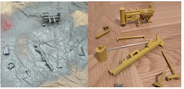
**Step 24:** Leave the primer coat to cure fully before applying the top coat. The correct paint code for Bryce Suma Yellow is RAL 1007. This can be purchased in a spray can from your local car body supply shop. Alternatively we have used Halfords Rover Inca Yellow which is a reasonable match that can be found at any Halfords shop.
