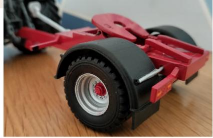
**Step 9:** For modern versions the mudguards are fixed by gluing along the mounting bracket and lining up with the two wires sticking out of the chassis. Touch up any paint where damaged or smudged by glue.
