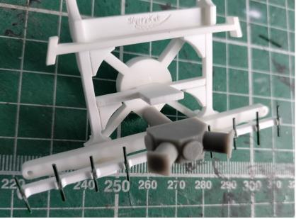
**Step Ten.** Add the diverter block as pictured. It should fit in the hole in 10 and the flat should glue onto the edge of 1.
