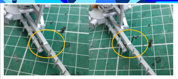
**Step Eighteen.** Begin final assembly by adding pins to the booms. Cut a length of 1mm wire. Bend one end up, thread through the boom and the pivot, then fold the other end up and trim to size.
