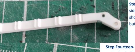
**Step Thirteen.** Peel the backing off both sides of the thin plastic parts. Glue the shorter one to the end of 2 as pictured butting it up to the first notch.
