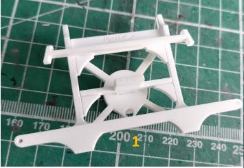
**Step Eight.** Glue 1 to the front of the assembly (your 1 will have slots in, don't worry.) Glue centrally and with the top inline with the fillet on 5
