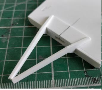
Glue the spare wheel mounts 23 back to back, then glue these to the offside front 10mm back from the front of the trailer.
