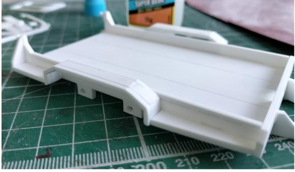
**Step Eight.** Assemble the ramps. Start by gluing a side 15 to the main ramp 16 aligning the top of the point with the end of 16.
