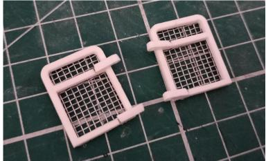
**7.** To fit the doors cut a length of pin wire (the thinner wire) and bend the end 90 degrees. Slot the pin down through the hinges and then bend the end to lock the pin in place, trim any excess wire.
