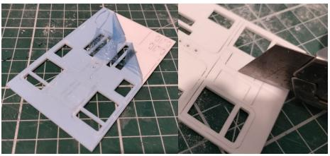
**1.** Remove the plastic film and separate the parts from the sprue by gently cutting through the remaining plastic. Sand all parts with 220 grit or similar sand paper.
