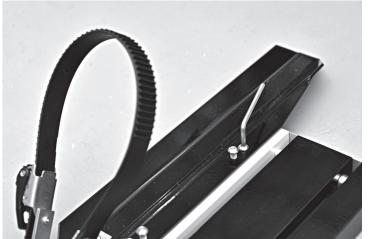
3. place the wheel holder on the corresponding rivet nuts of the base carrier (note right and left side) and tighten each with 4 screws (M6, 15 mm) with the spring washers using the supplied Allen Key (6 Nm).
