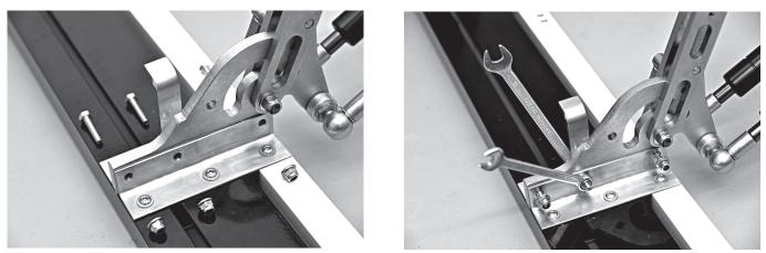
2. insert the 3 screws (M6x25 mm) through the holes and tighten them with the nuts (M6, self-locking) and the supplied combination spanners (10 Nm).
