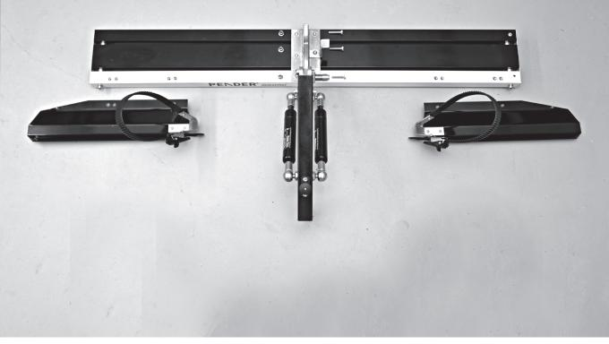
1. Insert the lifting mechanism into the angle plates of the base carrier so that the screws can be pushed through.
