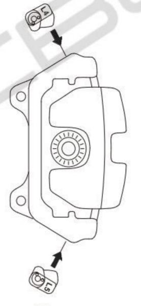
Step 2 Put caliper cover over the caliper
