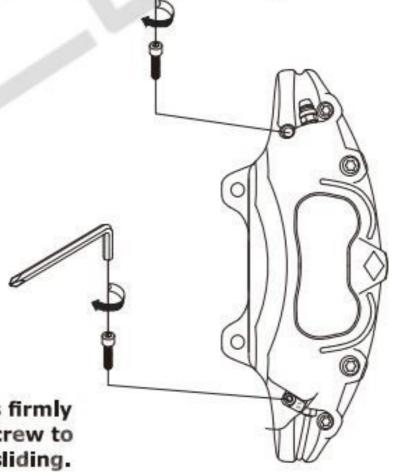
Tips: fasten buckles firmly when turning the screw to avoid rotating and sliding.
