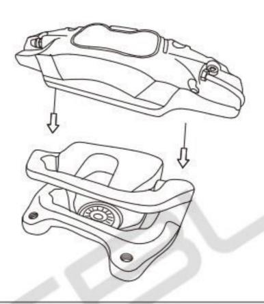
Step 3 Insert screw into holes shown as below, aligning R5, R4 buckles and then turning the screw
