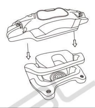
Step 3 Insert screw into holes show as below, aligning L4, L5 buckles and then turning the screw.
