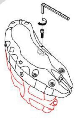
Model S/X Rear Left Caliper Cover Installation
