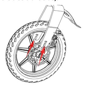
3. Straighten the folding stem and tighten the lock catch.
