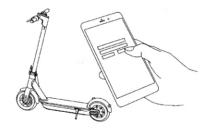
3 Click "Vehicle" → "Scan for Vehicle" to connect to your KickScooter. The KickScooter will beep when the connection is successful. The Bluetooth icon will stop blinking and remain illuminated.
