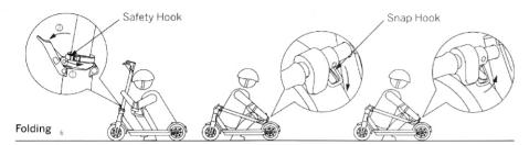
Turn off your KickScooter. Turn the safety hook counterclockwise and open the quick release lever.
