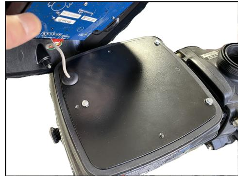
Figure 6 - Display Removed
