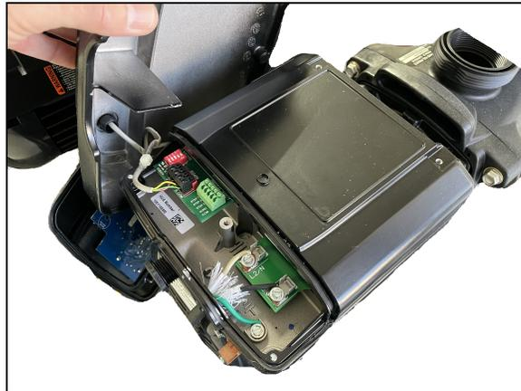
Figure 8 - Inner Cover Removed
