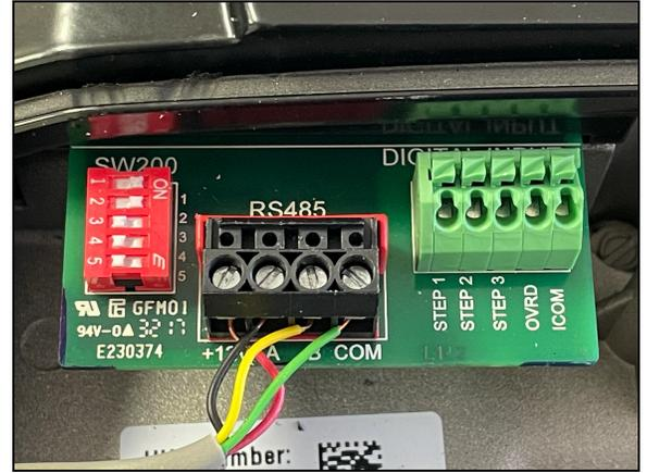
Figure 9 - Remove Existing Display Wires from Connector
