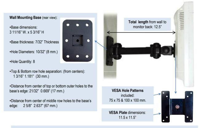
Load capacity recommended: for LCD monitors up to 22lbs (10 kgs.)
