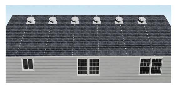
Placement of vents should be evenly spaced across the length of the roof.
