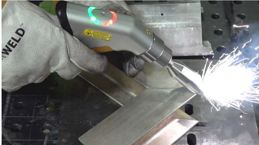
Aluminum I Beam (Clean & Weld) 0.25" (6 mm) Aluminum 6061
