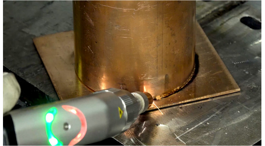
Welding 3 mm copper pipe to 2 mm flange
