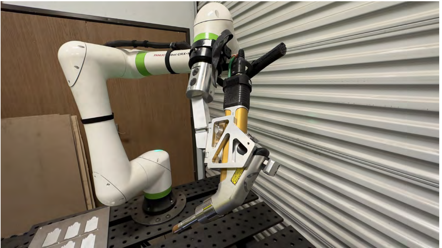
The IPG co robot gun holder uses the standard LightWELD GUN to allow safe control by the Fanuc CRX controller.
