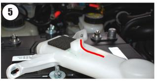
7). Insert battery hold down 'J' bolts into tray, place battery in tray, fit top mount, washers and wing-nuts. TIP: Use electrical or masking tape to hold J bolts in place against the side of the tray. Battery terminal posts are best located to the rear. (Refer Pic. 4)
