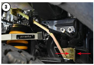
**4).** From under wheel arch, manenuver support arm up into position. It sits engine side of plastic arm off air filter housing. Slip backing nut plate into body crossmember box section and loosely fit all five M8 x 25 bolts. Ensure backing plate shim is located correctly (Refer Pic. 3)
