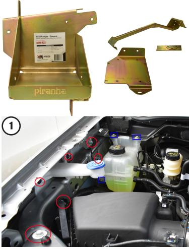
**3).** Check earth wire is sitting in the groove of the perimeter beam, refit original bolt and tighten. Tighten three coolant expansion mounting bolts if they were loosened previously.
