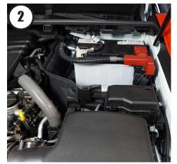
1). Unclip battery cover, remove the following items: Red plastic cover over positive battery terminal (including the plastic base the cover clips to) and positive lead off terminal that crosses the front of the battery (Refer Pic.2), battery foot clamp at Drivers Side front corner, remove battery, plastic battery sub tray, fibre heat shield beside engine.
