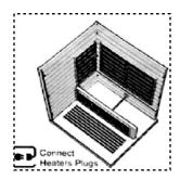
Connect the heater plugs under the bench to the appropriate sockets.
