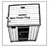
Slide the dust cover over the top panel and pass the main power plug through the opening. Make sure to match the holes for the vent on the dust cover with the sauna's vent holes.
