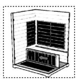
Before installing the right panel, you need to install the bench. Slide the bench stand panel between the two (2) vertical guides on the side panel.
