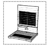
Place the back panel on the back end of the floor panel. At this point, someone should hold the back panel in place until at least one (1) side panel is connected.
