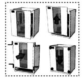
Connect the front panel to both side panels as per the image. Make sure to align the corners of the two (2) side panels and the edges of the front panel.
