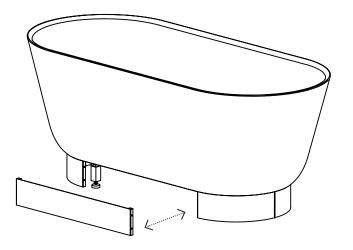
Remove the magnetic front panel to access the bathtub's technical space.
