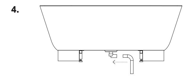
The installaton requires a separate drainpipe depending on the site. Drainpipe connector is for a 32mm (od) pipe.
