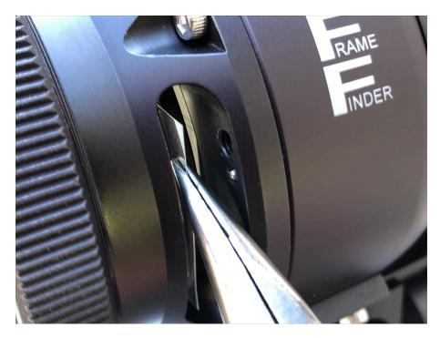
Then, looking into the front of the finder, center the frame-line pattern, left to right, and top to bottom, and adjust any slight rotation if necessary, occasionally checking the alignment by looking into the eyepiece. Once aligned, gently tighten the four Phillips-head screws in the corners of the frame.
