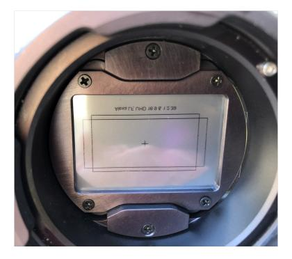
Using the #0 Phillips-head screwdriver, loosen those four screws, one full turn of rotation, in the corners of the frame, as seen in this photo. *There is no need to remove them.*
