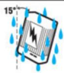
Protected against vertically falling drops of water with enclosure tilted up to 15 degrees from the vertical. Limited ingress permitted.
