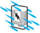
Protected against sprays of water up to 60 degrees from the vertical. Limited ingress permitted for three minutes.
