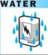
Protected against vertically falling drops of water. Limited ingress permitted.
