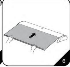
6.Hold the graphic and allow it to recoil into the base unit.
