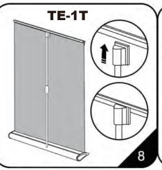
8. Lift the graphic and make it fixed onto top of the pole.
