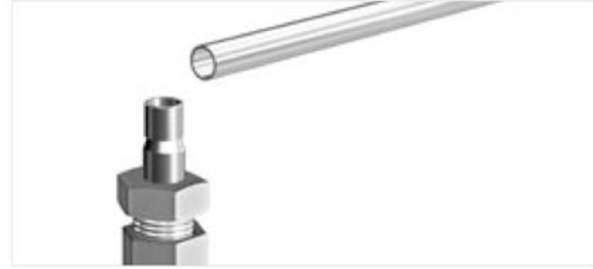
3. Connect Male Tube adapter to female port.
