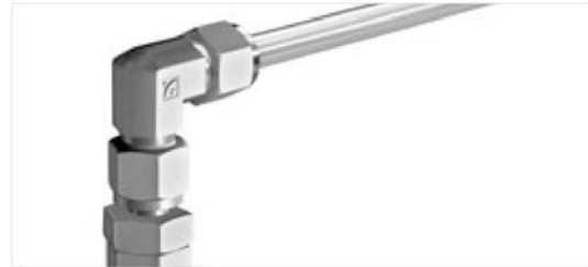
4. Connect union elbow to adapter by tightening SUPERLOK connection with wrench while holding elbow pointing in desired direction. Then insert tubing into the other end of the Union Elbow and make up fitting.
