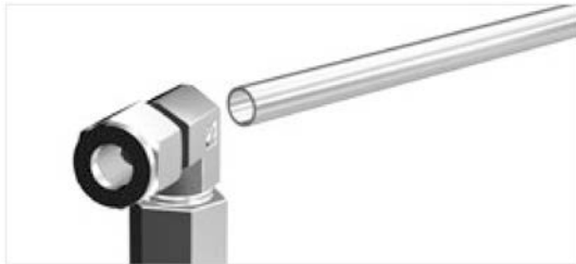
2. With pipe connection tight, the male elbow is pointing in the wrong direction for desired tubing run.
