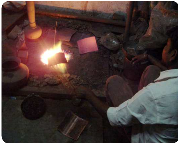
Sheets of copper are heated on the coal fire till they turn red hot. This makes the copper sheet malleable so that it doesn't split or break while it is being beaten into shape. The copper sheets are available in different thicknesses generally between 8 gauge - 16 gauge. Also they are not pure copper but a 80/20, 50/50, 40/60 mixture. Pure copper is heavy, expensive and more malleable. Traditionally pure copper was used however now utensils from pure copper are only made when they are made by braking down old utensils.
