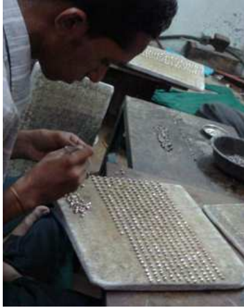
Individual patterned loops of an anklet are placed in rows on an asbestos sheet for welding.
