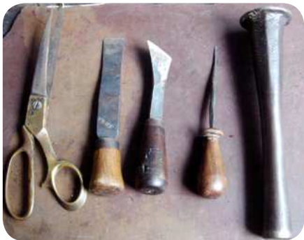
The awl is a pointed tool with various purposes- to pierce holes through which threads can be drawn and to join the shoe upper and sole together.
