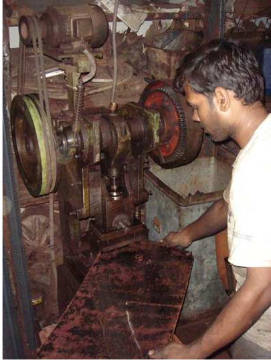
The metal sheet cut into the required sizes is punched on a punching machine.
