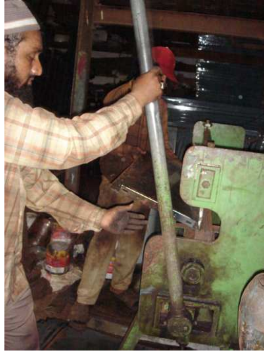
The edges of the sheet are folded over at right angles.
