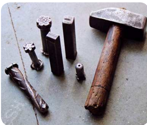
Metal dies with various patterning are available. They are used to imprint the leather with decorative designs by hammering them onto the leather surface.
