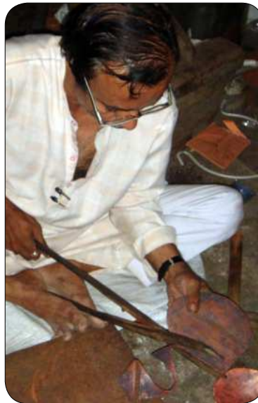
The sheet is cut into a circular shape. It is easier to cut when it has been recently taken of the fire.
