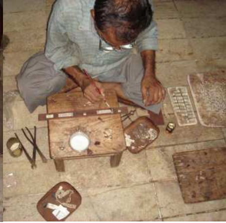
A white solution is applied to the different pieces of an anklet at their point of attachment.
