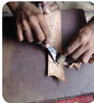
A flat sharp chisel is used to scrape away the fibrous excess from the underside of the leather piece making it smooth.
