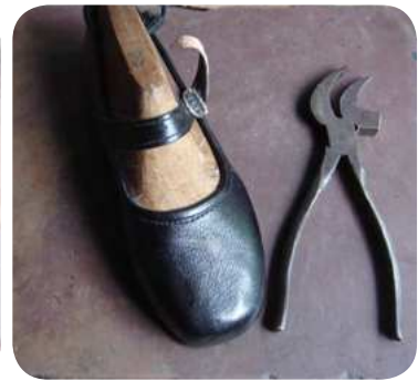
The last (left) is the form used to shape the upper and lasting pincers (right) are used to pull the upper leather right around the last before it is secured with tacks.
