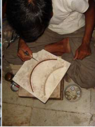
Different patterned silver pieces are arranged on an asbestos sheet to be welded together into a neck ornament.
