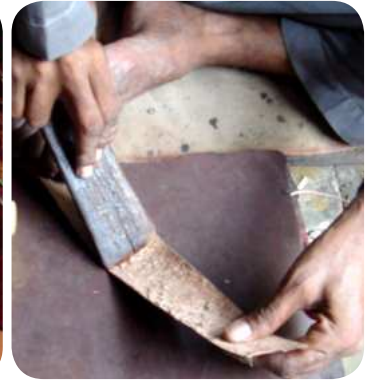
The khurpaa is the most important tool. It is used to etch out the required shape onto the leather. Also to stretch and pull the leather into shape.
