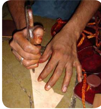
The khurpaa is the most important tool. It is used to etch out the required shape onto the leather. Also to stretch and pull the leather into shape.
