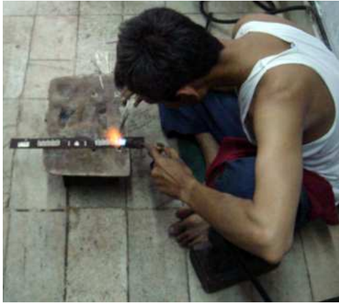
The arrangement of silver pieces is then welded together.
