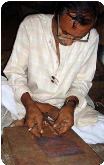
A circle is etched onto the sheet using a metal compass.
