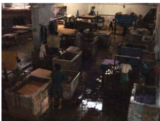
(Above) cotton pulp being converted into sheets of paper. (Left) sheets of paper hung to dry.
