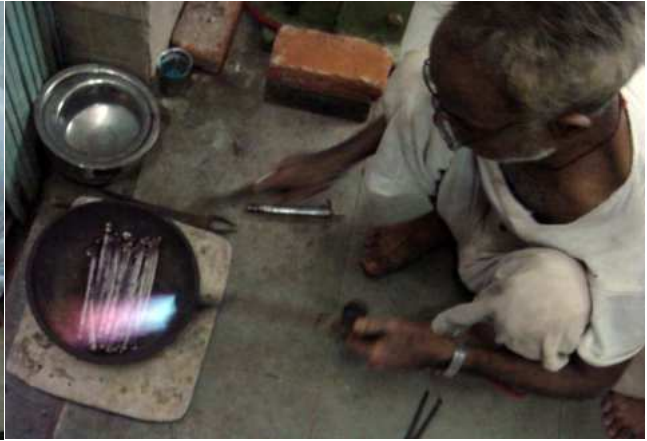
The ready pieces of silver ornaments are then treated to a flame for about 2-3 minutes. They are then washed in sulphuric acid solution. This is done to polish the silver and give it lustre.
