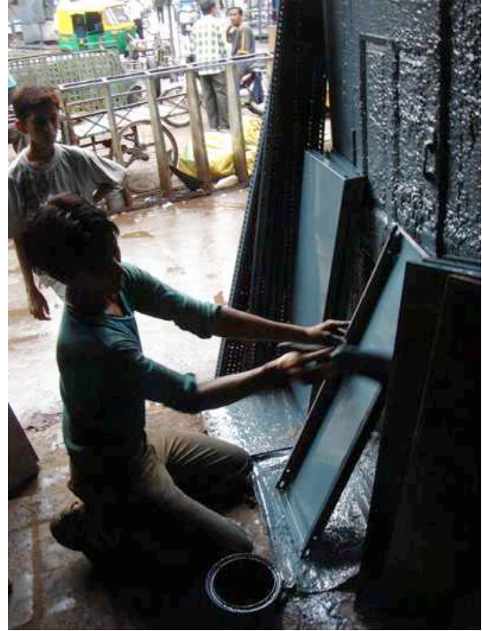
Finally the individual pieces are painted before being joined together.
