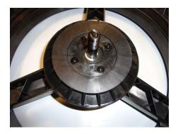
Ensure the Brake Disc is seated so that it does not spin.
