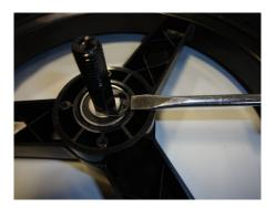
WEAR SAFETY GLASSES WHEN ADDING E-ECLIPS! Use Plyers, or a Flat Head Screwdriver, to add the E-Clip.
