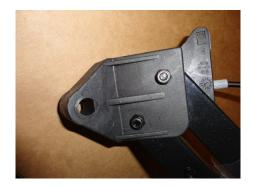
Attach the Brake Housing to the Brake Housing Adaptor using a 10MM Open End Wrench, the remaining Rectangle Head Screw (SV1-208), and two M6 Nylon Nuts.
