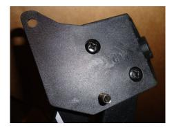
Insert a Rectangle Head Screw (SV1-208) into the inside Rectangle slot of the Brake Housing Adaptor, as shown.
