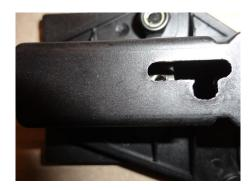
Put the Brake Lever in the 'Brake On' (Down) position. Twist the Brake Pin until you can see the threads in the Brake Pin.
