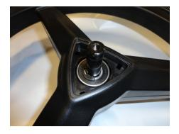
**WEAR SAFETY GLASSES WHEN ADDING E-ECLIPS!** Add an E-Clip to inner slot of the Cap Side of the Front Axle. Install the Front Axle with the Cap Side out of the Deep Cavity of the Front Wheel.
