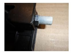
Brake Cable Adjust Studs.
