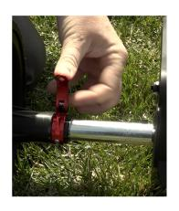
6) Finally, push your front and rear wheels in by opening the cam lever on each axle, pushing the wheels in and refastening the cam levers. Now, the wheels are all locked in place.
