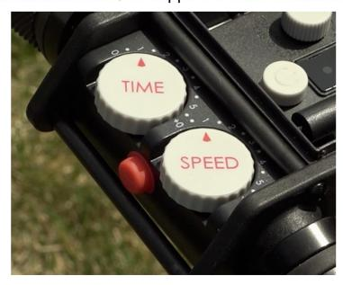
This cart has a feature which allows you to use it without the use of the remote. On the top of the tray you will see two knobs, the one on the left controls the time the cart will run and the knob on the right controls the speed. Start with both of these knobs on a low setting to understand how fast and far the cart will go on each setting. With the two knobs set to low settings and with the cart in an open area, simply push the red button beneath the two knobs and the cart will go.
