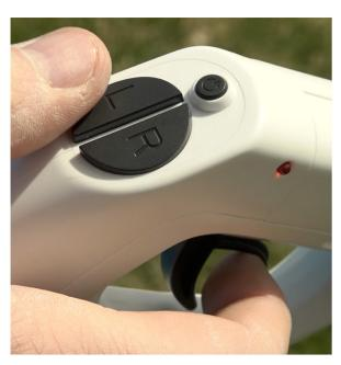
2) The two buttons on the top of the remote allow you to turn the cart right and left by simply pushing them with your thumb.
