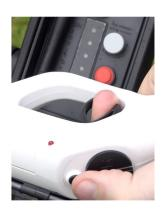
2) Next grab the remote, pull the trigger all the way back and power on the remote. You will hear a ding and the lights in the tray will blink slowly.
