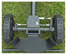
2) When the front wheels turn, adjust the tracking with the gray button in the tray until the wheels are straight.
