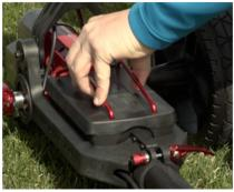
2) Now, raise the body of the cart and the tension bar, open the lower bag support, release the cam lever so you can pull the front axle out and insert the battery.
