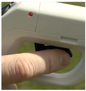
1) Pulling back on the trigger makes the cart go forward and pushing forward on the trigger engages reverse. The cart will slow to a stop by simply releasing the trigger. If you need the cart to stop quicker push the trigger completely forward. Please note, if you use this method you will need to fully release the trigger and press forward again for the cart to engage reverse.
