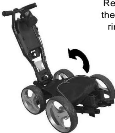
Release the folding latch underneath the accessory tray by lifting up on the rim of the cup holder. While holding the front wheel in place with your hand or foot, pull the handle back until the upright tubes are fully extended. Secure the cart by engaging the yellow latch hook and lever as shown in the illustration on page 4. If your lever is too tight, loosen the nut at the base of the latch hook,
