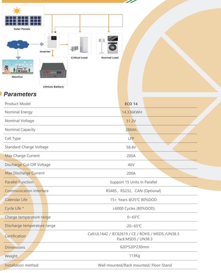
\*Test Condition: 80% DOD, 0.2C charge & discharge @25°C
