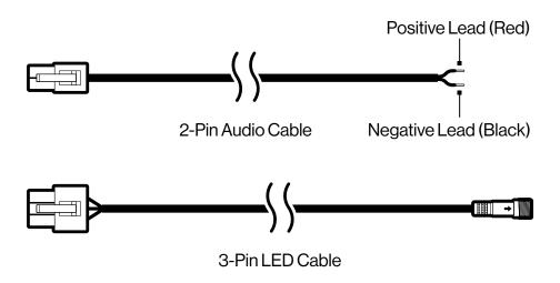
5. Plug in the Audio Cable into the 2-pin Audio Jack and the LED Cable into the 3-pin LED Jack on the speaker.
