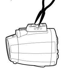
or similar tool. Failing to do this will result in potential water or moisture penetration into the jack connector pins, causing damage to the speaker and **VOIDING THE PRODUCT WARRANTY**.
