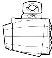
· Locking Screw Latch with a Hex Nut – It is necessary to use an Allen wrench (included) to tighten or untighten the latch.
