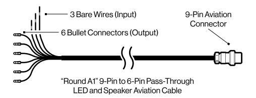
• The long cable ("Round A1" 9-pin to 6-pin pass-through Aviation Cable) has a 9-pin round connector on one end and 3 bare wires for power inputs and 6 Bullet connectors on the other end for interconnection with the Passive Tower Speaker.
