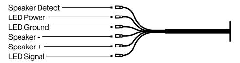
The Passive ExtremeTower Speaker only has 6 input wires.
