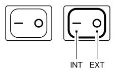
3. Open the Back Cover (refer to **Install the Rechargeable Battery Pack to the Amplified Speaker** for details), move the (Blue) FM ANT Switch to the EXT position.
