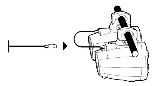
4. Plug in the 4-pin Deutsch Power Cable's connector into the 4-pin Deutsch Connector Jack on the Amplified Speaker.
