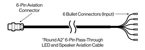
• The short cable ("Round A2" 6-pin pass-through Aviation Cable) has a 6-pin round connector on one end and 6 bullet connectors on the other end.
