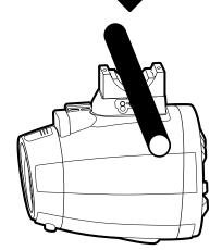
11. Turn the speaker to your desired angle, tighten the Locking Screw with the supplied M5 Allen wrench (or with your hand if utilizing the Quick-Release Knob).
