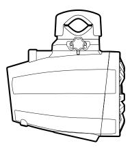
Locking Screw Latch with a Quick-Release Knob – A tool is **NOT** required to tighten or untighten the latch.
