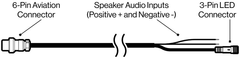
“Round C” 6-Pin Pass-Through LED and Speaker Aviation Cable
