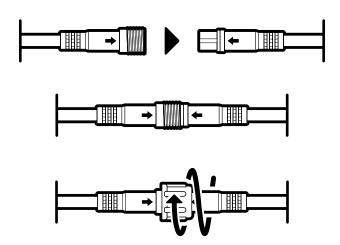
2. Connect the 3-pin male connector on the LED Control Cable to the LED control output 3-pin female connector on a SoundExtreme product with LEDCast technology.
