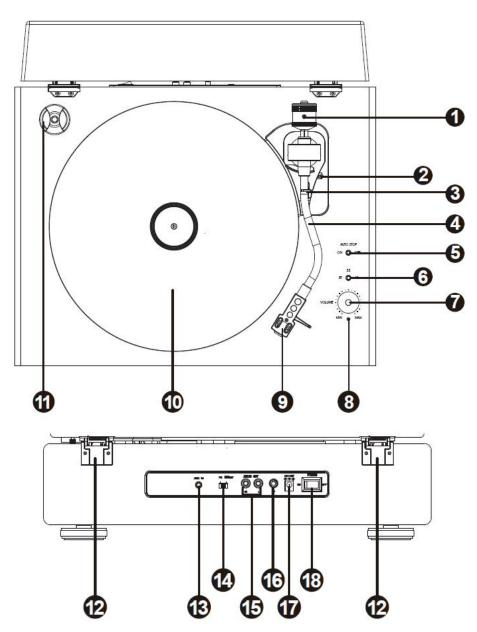
1. Tonearm Counterweight—adjust the counterweight to make sure that the needle pressure is at 3G, +-0.5G measured by a needle balance(not included in the package)
