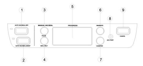
AUTO VAC/SEAL-DRY: At stand-by condition, it starts the automatic operation of vacuuming the bag and then automatically seals the bag when the vacuum is complete; this function for dry bags and items without moisture with a shorter heat sealing time.
