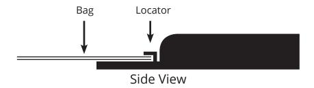
It is vital that the top of the bag is correctly located with the full width of the bag **inside** the bag locator. Failure to locate the bag properly is the most common cause of problems with Lava machines.
