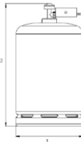
Key 1 "Maximum diameter or breadth".... 2 "Maximum height (regulator included)."...
