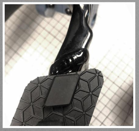
**5° PASSO:** REMOVER A PELÍCULA E POSICIONAR O PROTETOR PRÓXIMO A SOLDA, CONFORME MOSTRADO NA FOTO.
