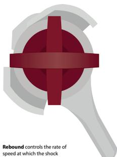
**Rebound** controls the rate of speed at which the shock extends after compressing.
