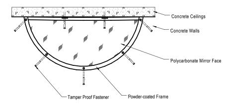
NOTE: If installing with Rawl Spikes, it is recommended to use a punch. This is to eliminate damage to the mirror and powder-coated frames.
