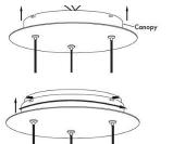
Twist canopy to lock fixture in place. Secure canopy with canopy screws (F).
