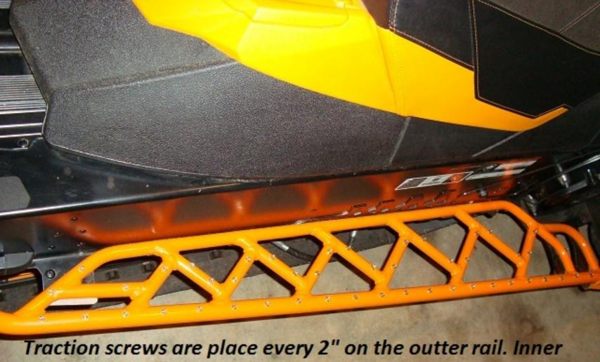
Traction screws are place every 2" on the outter rail. Inner tube locations are all approximate. Place where desired. 50 are supplied for each side. Drill 1/8" pilot hole then screw in. Enjoy your new Burly Boards!!
