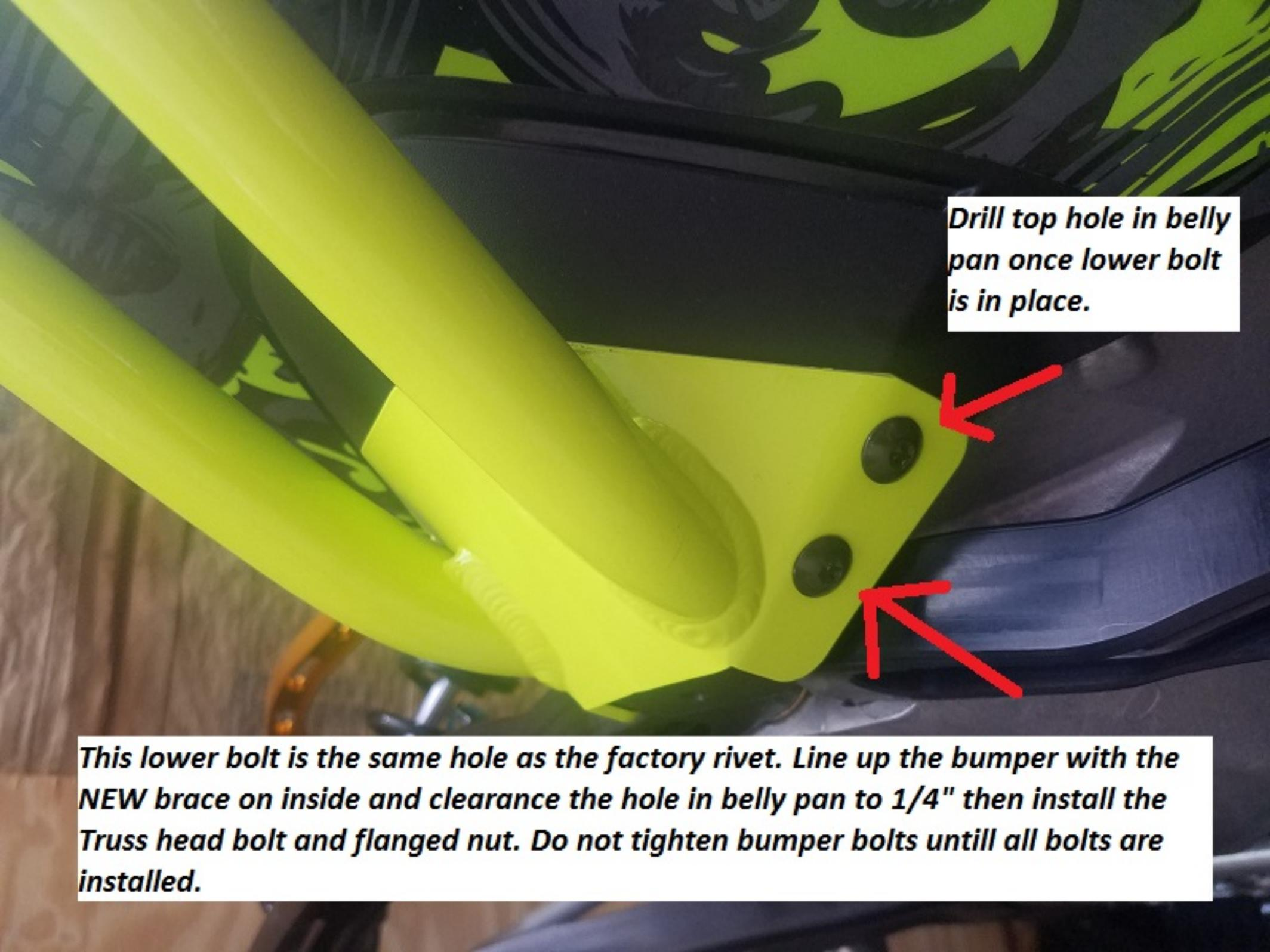
A close-up photograph of a motorcycle bumper assembly. The bumper is a bright yellow plastic component with two circular holes. Two black bolts are already installed in these holes. Two red arrows point to the bolts. The bumper is mounted to a dark grey metal frame. The background shows a wooden floor and a black plastic fairing with a green and black graphic.
