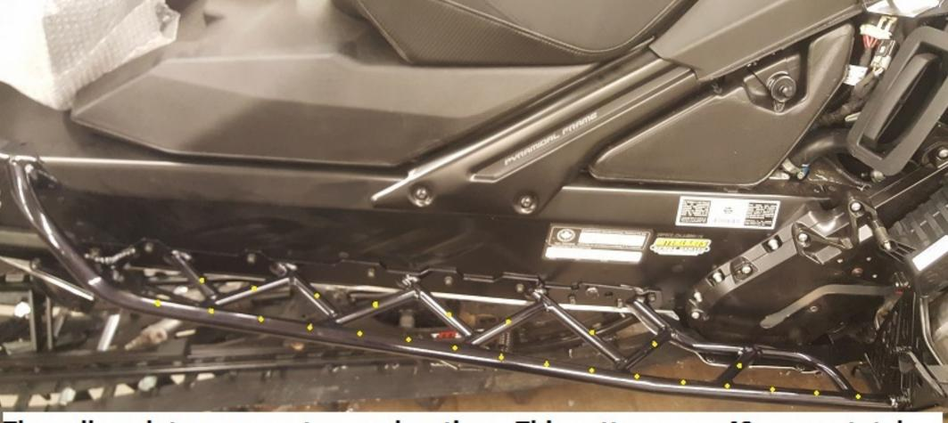
The yellow dots represent screw locations. This pattern uses 48 screws total, 24 each side. You may want to add more towards the front of the board. We start with the minimum and add more as needed.
