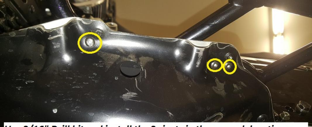
Use 3/16" Drill bit and install the 3 rivets in these rough locations.
