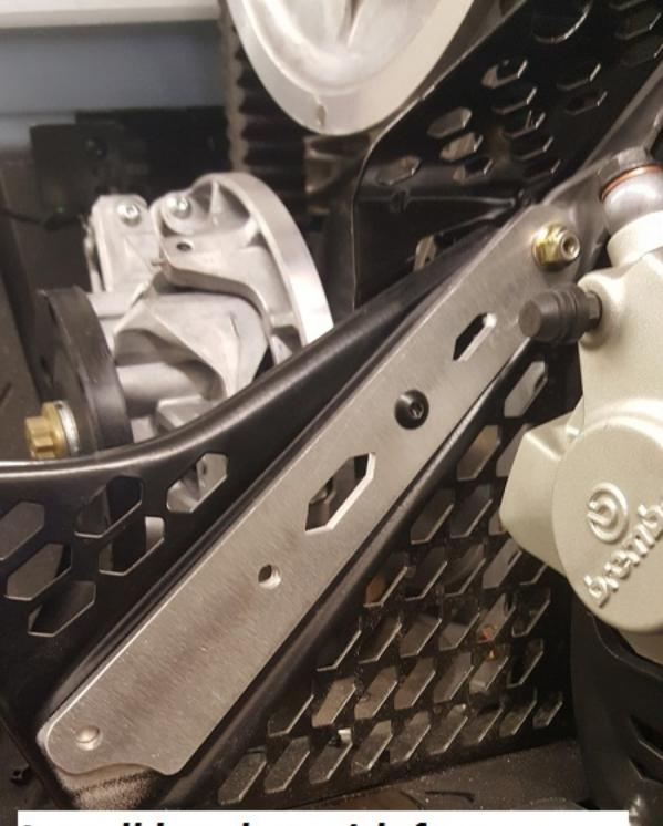
Install bracket with factory hardware. Note the orientation of the bracket. Align the holes and tighten. Shown raw for clarity.
