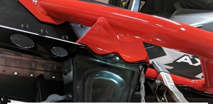
Clamp the board in multiple places along the tunnel. Align the rear mount as pictured. The front hoop of the board should align as shown in pictures below. The 3 factory rivet locations in the rear suspension hanger need to be equally spaced onto the board. These will be bolted down with the supplied 3/4" long button head bolts and flanged nuts. Use a 1/4" bit to drill the holes.
