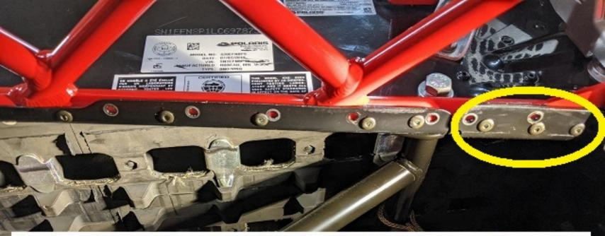
The 3 rivets circled here need to be the LONG rivets the rest are still the short ones. There is two layers of tunnel here the needs the long rivets. Mark there locations as shown.
