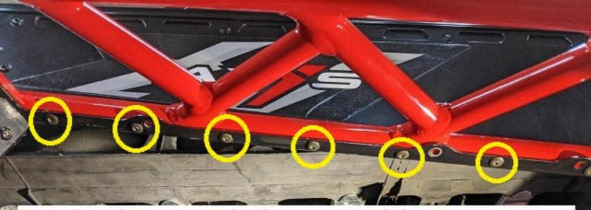
Rivets shown here are spaced 2.5" apart, start with the rear most one placed roughly 1/2" forward of rear hangar. Mark rivet locations to layout as pictured. Be sure to keep board clamped tight to tunnel as you drill and install the rivets. Use the <u>short</u> rivets supplied here. Rivet must hit the center of the tube. Take your time.
