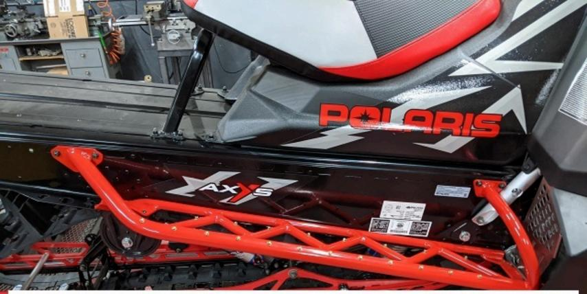
Final Step! Install traction screws. Use a 1/8" drill bit first, then use an impact driver to run the screws in. The screws shown on the outer rail are spaced roughly 2.5" apart and only 1 screw per inner tube. We recommend starting out like this. You may have a different preference. Remember, only 80 screws are supplied.
