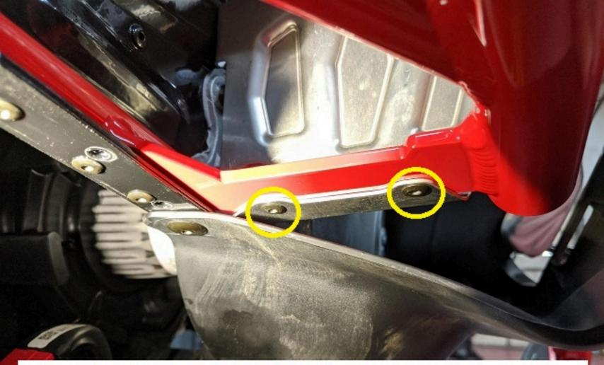
Drill and install 2 short rivets holding the toe plate onto the board. Circled in yellow. Reinstall the large head rivet holding the belly pan on. Arrow indicates this location.
