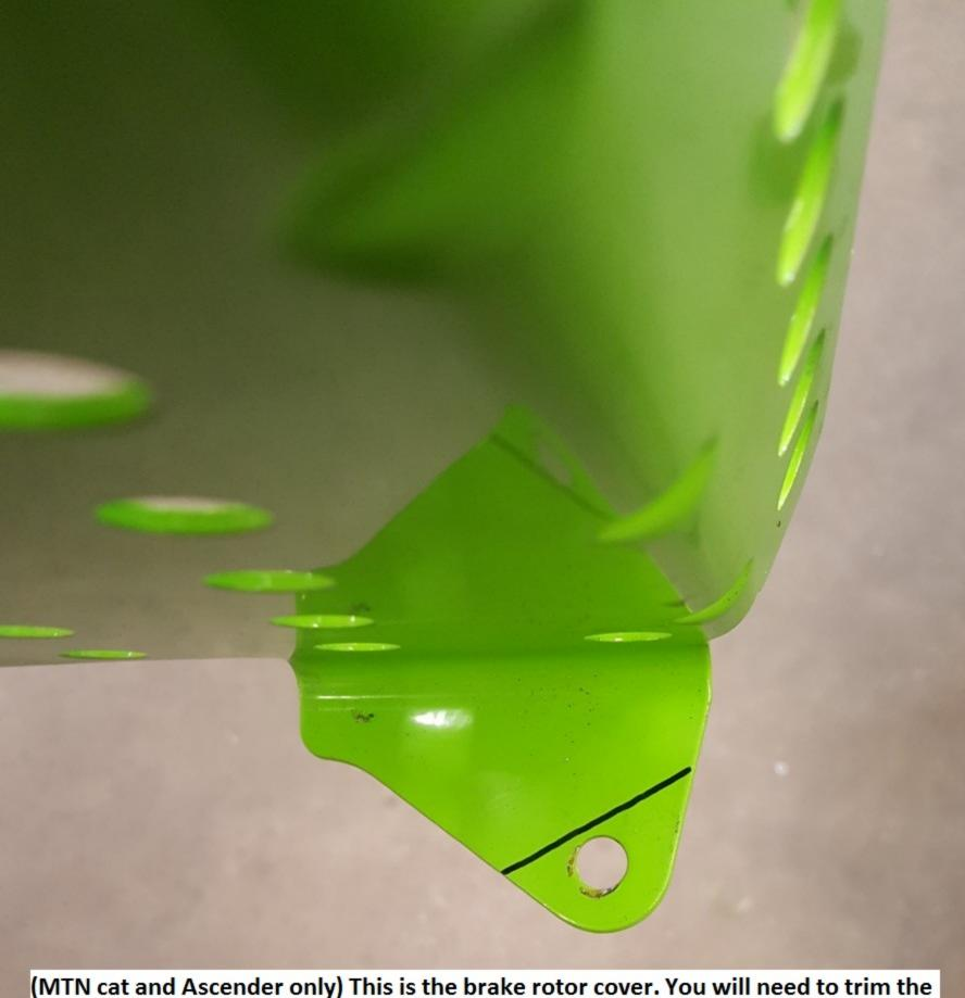
(MTN cat and Ascender only) This is the brake rotor cover. You will need to trim the mounting ear as shown so it will clear the board. Once trimmed, re-install and find a correct spot to drill a new mounting hole from the bottom up. Use the factory bolt and spring clip to attach. (Can be seen in picture of plastic lower rotor cover circled in BLUE)
