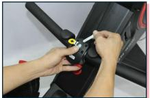
While keeping thumb on cover, remove battery cover with a small flat-head screwdriver.
