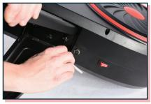
2. Tighten the screws with hex key.
