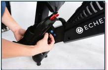
12. Align the right foot carriage with the screw holes on the body of the rower and hand tighten the three screws.
