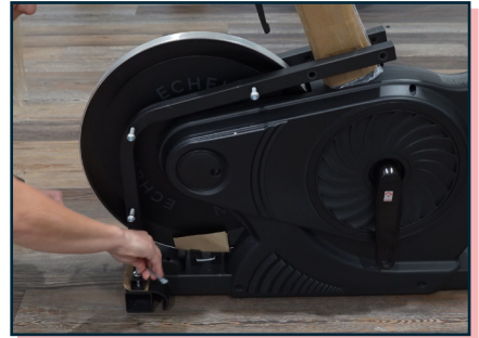
Remove bolts on both sides with included tool as shown.
