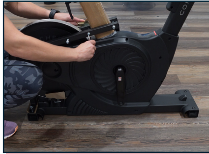
Remove bolts with included tools as shown.
